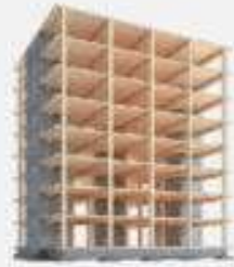
Timber 5 Timber Post, Beam & Plate; Concrete Cores
